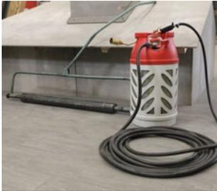
The following is used in the work: a big and a small torches, a metal holder for rolls' unrolling and an assembled gas cylinder. At the start, it is necessary to set up the equipment, check the integrity of hoses, examine the operability of LPG pressure regulator and the integrity of the junctions.
