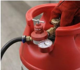
When igniting a propane gas torch, one should turn the valve from a quarter to half a turn, and after a short gas blowing, ignite the burning mixture and then adjust the length of the flame.
