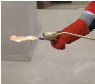
A torch is ignited with a match or a special lighter. It is forbidden to ignite a torch by means of random burning items. One should not walk with a burning torch beyond the borders of a working place, climb the ladders and scaffolds, or move abruptly.
